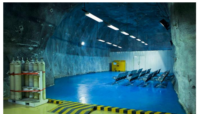
200 Persons Permanent Refuge Chamber developed at Freeport McMoran , Indonesian Mine
