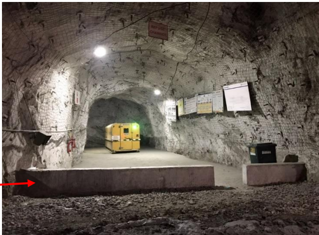
20 Seater Refuge Chamber installed at Kayad Mine, HZL
